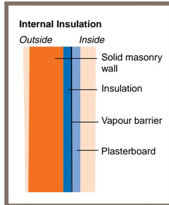
Types of insulation material used include expanded polystyrene, fibreglass and polyurethane boards. Polyurethane tends to be more expensive, but its thermal performance is approximately 50% better than polystyrene or fibreglass, so a 25 mm (1 inch) thickness of polyurethane will have roughly the same insulating performance as a 38 mm (1.5 inch) thickness of polystyrene.
