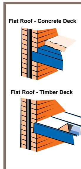
If you have an existing flat roof, insulation can be increased externally with extruded polystyrene or foamed glass, or internally with an insulated lining board such as mineral fibre or polyurethane foam-backed plaster-board.
