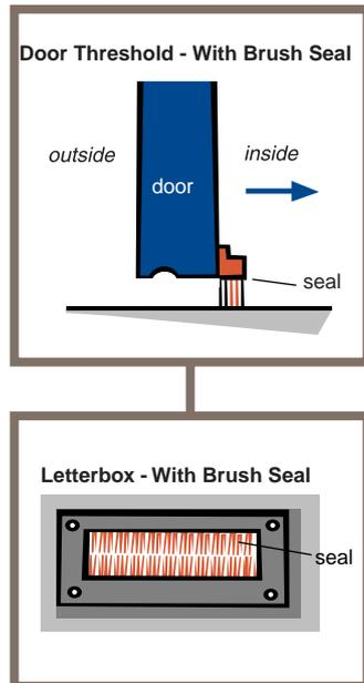
Letterboxes with just one inward-opening flap will tend to admit draughts, particularly when the wind is blowing directly on the front door. Brush seals are commonly used to reduce draughts through this type of letterbox.
