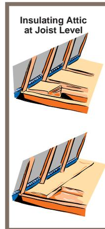
After the attic is insulated at joist level, its temperature is reduced, so you must insulate the water storage tank and pipes.
